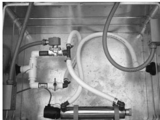
The manufacturer of the commercial UV unit does not recommend intermittent use of the system because it decreases lamp lifetime. But, because the BYOW system is used for much less than 24 hours per day, it is predicted that the trade-off in duration will favor the BYOW application. Additionally, the effect of a recommended warm-up time of the UV unit is being investigated for further BYOW iterations, and possible changes to BYOW operating procedures.
