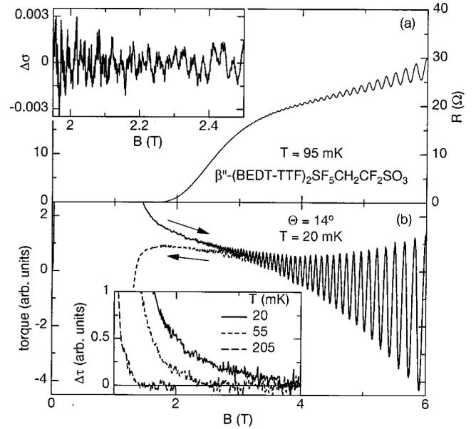
FIG. 2. (a) Field dependence of  $R$  and the SdH signal (inset) of sample *B* at  $T = 95$  mK. (b) Torque signal of sample *D* for up and down sweep. At about 3.4 T a clear hysteresis is visible. The inset shows the torque difference,  $\Delta\tau$ , for up and down sweeps at different temperatures. The irreversibility field is defined by the field where  $\Delta\tau$  becomes zero.
