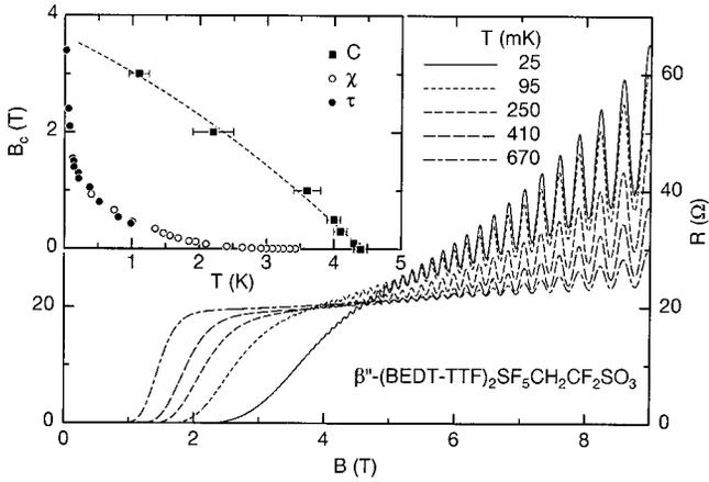
FIG. 1. Field dependence of the interplane resistance for selected temperatures (sample *B*). The inset shows the temperature dependence of the upper critical field as deduced by specific heat,  $C$  and the irreversibility field as extracted from susceptibility,  $\chi$  (Ref. 13), and torque,  $\tau$ , data. The dashed line is a quadratic fit through the  $C$  data and extrapolates to  $B_{c2} \approx 3.6$  T.
