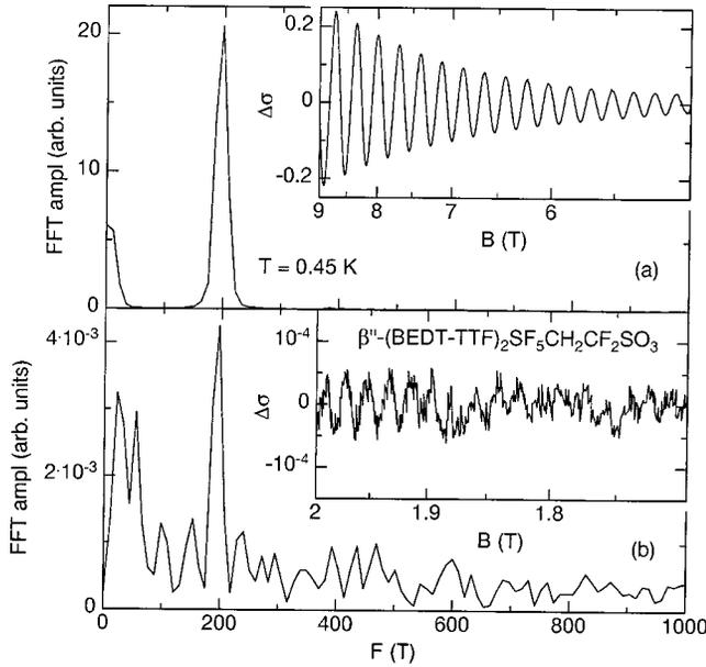
FIG. 3. Fourier spectra of the SdH signals (insets) of sample A at  $T = 0.45$  K in (a) the normal state ( $5 \text{ T} \leq B \leq 9 \text{ T}$ ) and (b) in the superconducting state ( $1.7 \text{ T} \leq B \leq 2 \text{ T}$ ). The  $x$  axes of the insets are scaled linear in  $1/B$ .
