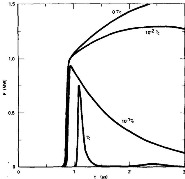
FIG. 4. Output power of a CO<sub>2</sub> laser with a 5:5:90 gas mixture of CO<sub>2</sub>:N<sub>2</sub>:He. The gain and loss coefficients are  $g_c = 1.5 \times 10^8 \text{ s}^{-1}$  and  $\gamma_c = 1.7 \times 10^7 \text{ s}^{-1}$ . As the loss is reduced the tail of the pulse changes, but the important leading edge and pulse delay are only slightly affected.
