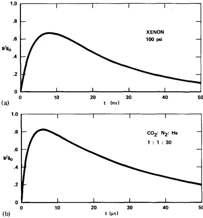
FIG. 1. Time-dependent gain functions for (a) a high-pressure electron-beam-excited xenon laser and (b) a resistive-pin TEA CO<sub>2</sub> laser. The xenon data is from Ref. 7, and the CO<sub>2</sub> curve agrees with the experimental results of Ref. 8.
