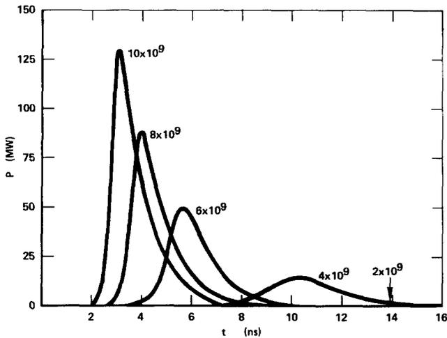
FIG. 2. Output power characteristics for a 1700-Å xenon laser as a function of initial unsaturated gain. The arrow marks the location of the small power maximum for  $g_c = 2 \times 10^9 \text{ s}^{-1}$ . Experimental results of Ref. 7 correspond approximately to the curve  $g_c = 4 \times 10^9 \text{ s}^{-1}$ .
