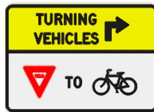
Figure T.5: Experimental level one: ODOT OR10-15b “Turning Vehicles Yield to Bicycles”
