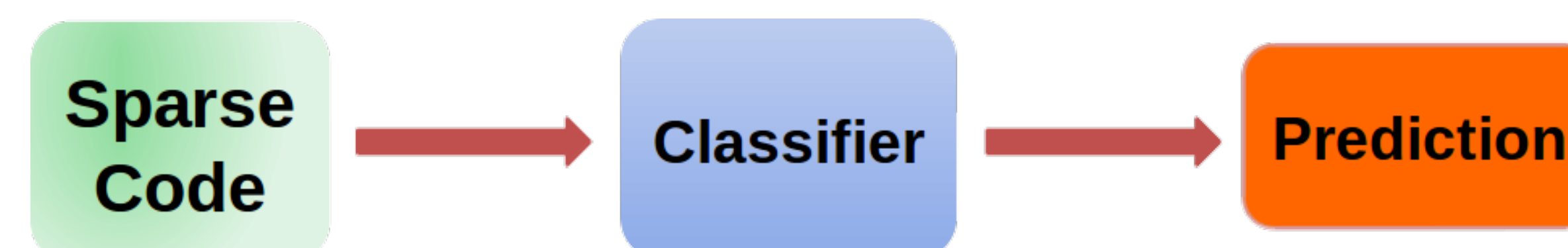
Fig. 4: The classifier portion of the procedure, at a high level. For a given image, the LCA produces a sparse code and passes it to the sigmoid layer. Each of the ten neurons are trained to fire for their respective class of digits such that one neuron fires for each image presented to the network.
