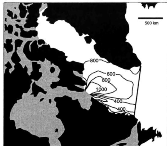
**Figure 4.** Steady state ice shelf thickness. Because most of the ice floats below sea level, this map can be viewed as an inverted map of basal topography. Large basal gradients in the Labrador Sea ice shelf are the basis for the Heinrich event mechanism proposed in the text. Basal melting is expected along the deep central keel of the shelf, while basal freezing is expected upslope along its flanks. The isopach interval is 200 m.
