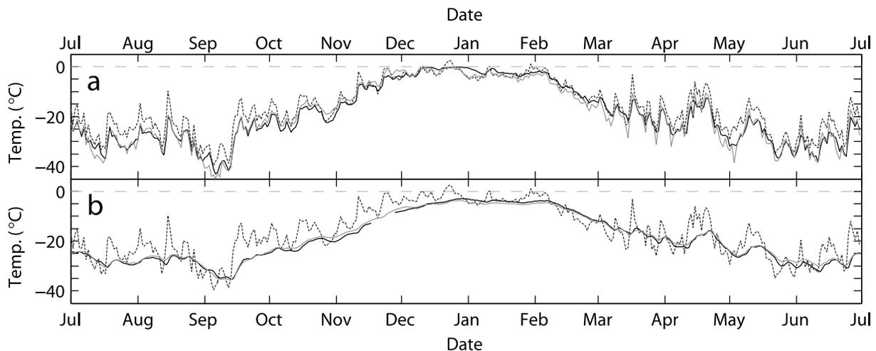
**Figure 6.** Measured (black line) and modeled (gray line) ice temperature and measured air temperature (dashed line) during model year 1995 for (a) the shallow thermistor (depth ablated from 12 cm to surface during this time period) and (b) the deep thermistor (depth ablated from 92 to 78 cm).
