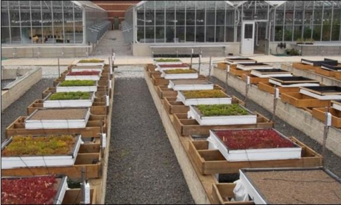
Figure 1. Experimental green roof platforms
