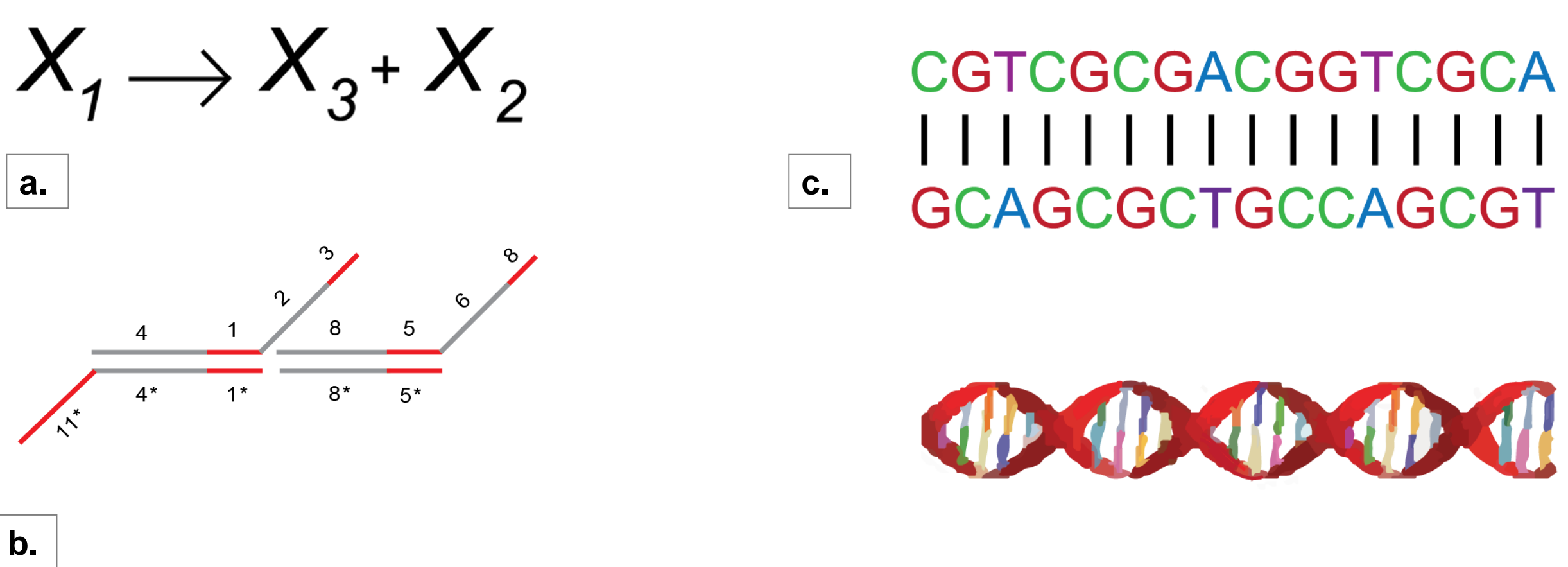
Fig 5. Reservoir networks as dynamic systems approximators of CRNs. The reservoir computing architecture is ideal for mapping to chemical reaction networks (a), which can be thought of as dynamic systems and can be described in detail using DNA domains (b) sequences and molecules (c). DNA molecules are desirable for parallelism and base-pair properties and avoid the limitations of a traditional semiconductor material such as silicone. Soloveichik et. al have also shown that DNA molecules "can be constructed that closely approximate the dynamic behavior of arbitrary systems ... " [4].
