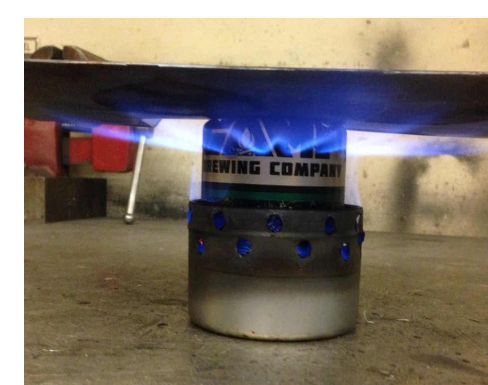
Fig. 6: Base Camp Burner in Container Store Base
