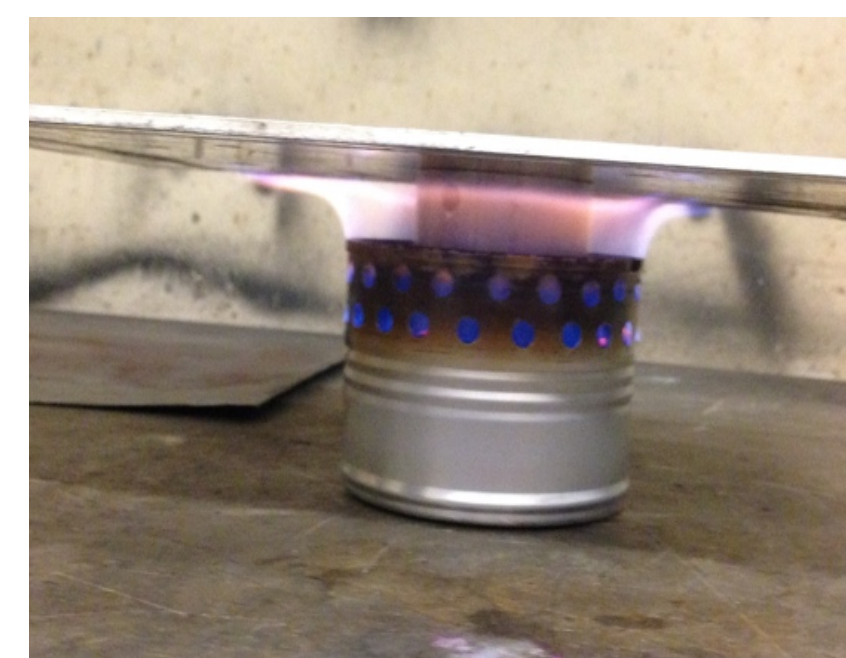
Fig. 4: Burner used in the 2016 Iditarod Cooker
