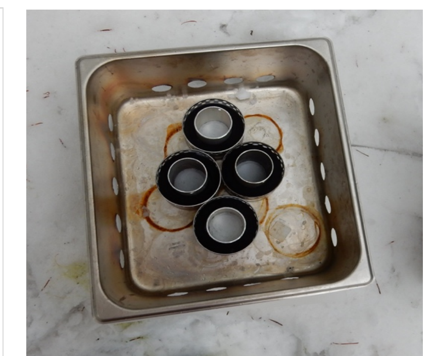
Fig. 9: Burner arrangement used during test on Mount Hood. Each burner held 100mL of HEET.
