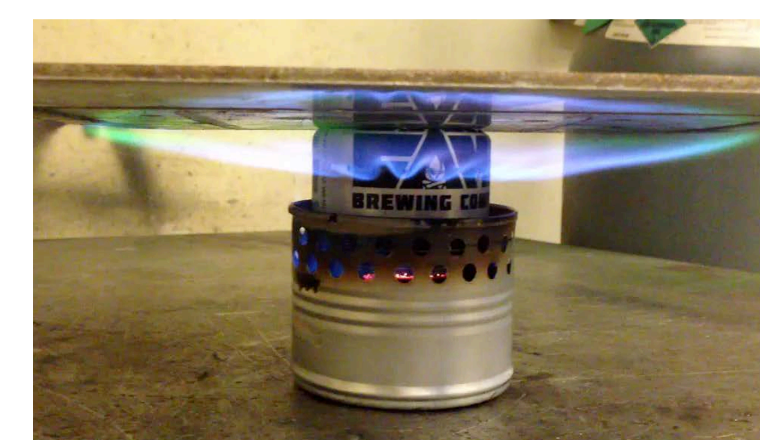
Fig. 8: Base Camp Burner with Vienna Sausage Can Base
