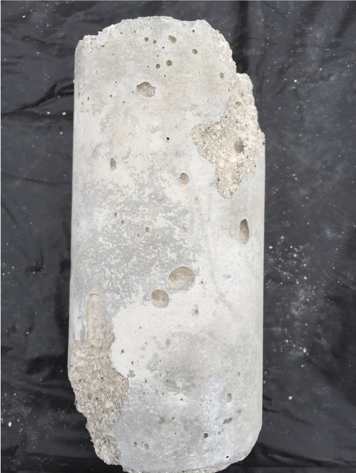
Figure 15: Type 5 Cylinder Failure
