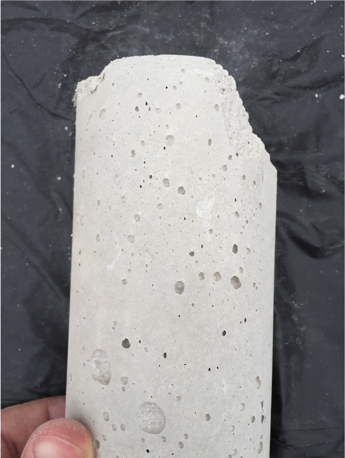
Figure 16: Type 6 Cylinder Failure
