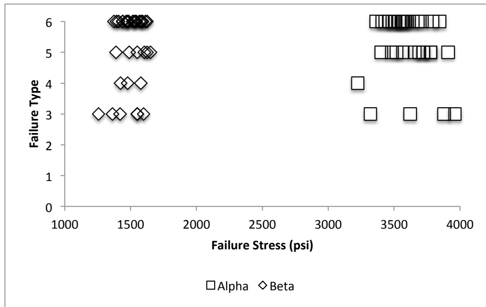
Figure 12: ASTM C39 Failure Type vs. Failure Stress
