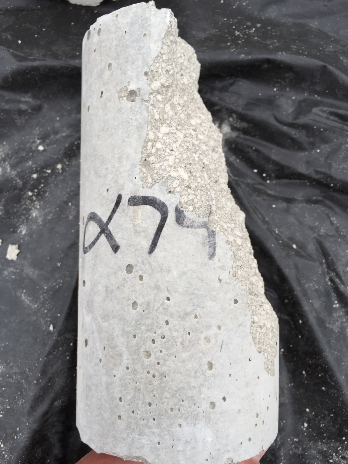
Figure 14: Type 4 Cylinder Failure
