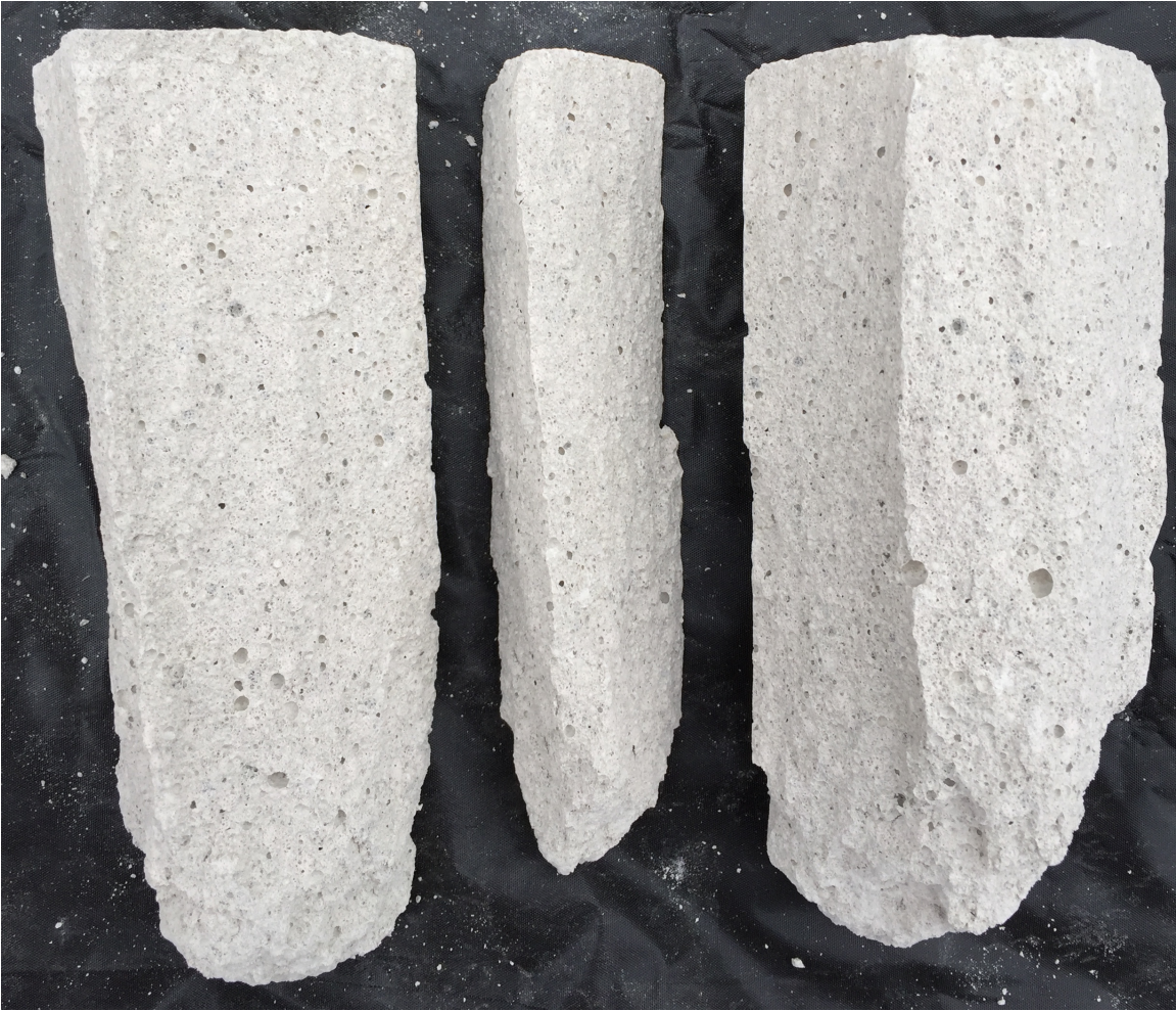
Figure 13: Type 3 Cylinder Failure
