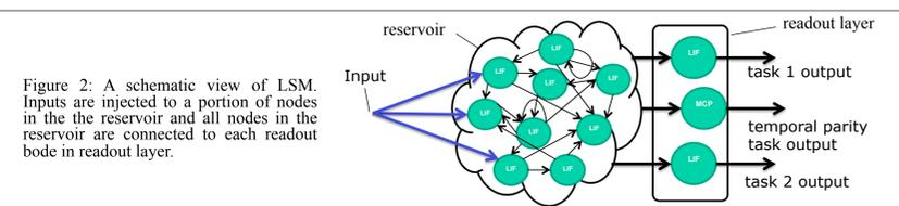
Figure 2: A schematic view of LSM. Inputs are injected to a portion of nodes in the reservoir and all nodes in the reservoir are connected to each readout node in readout layer.
