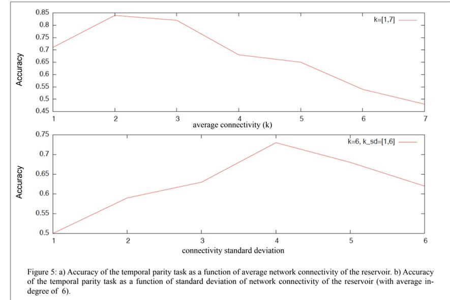
Figure 5: a) Accuracy of the temporal parity task as a function of average network connectivity of the reservoir. b) Accuracy of the temporal parity task as a function of standard deviation of network connectivity of the reservoir (with average in-degree of 6).
