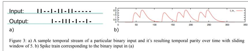
Figure 3: a) A sample temporal stream of a particular binary input and it's resulting temporal parity over time with sliding window of 5. b) Spike train corresponding to the binary input in (a)
