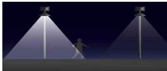
Figure 4: Streetlight sensors will only display full brightness when a pedestrian or car is near.
