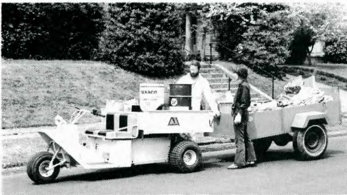
Figure 1: The Alsport UT-10 with trailer (10 hp., 1000 lb. total capacity, $2,300 from Alsport, Inc., 84 Whittlesey Ave., Norwalk, OH 44857)
