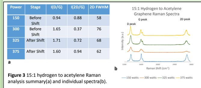
Figure 3 15:1 hydrogen to acetylene Raman analysis summary(a) and individual spectra(b).
