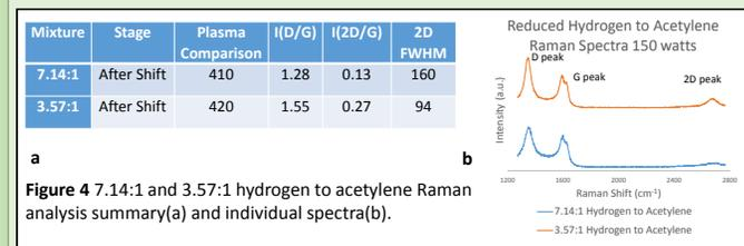
Figure 4 7.14:1 and 3.57:1 hydrogen to acetylene Raman analysis summary(a) and individual spectra(b).
