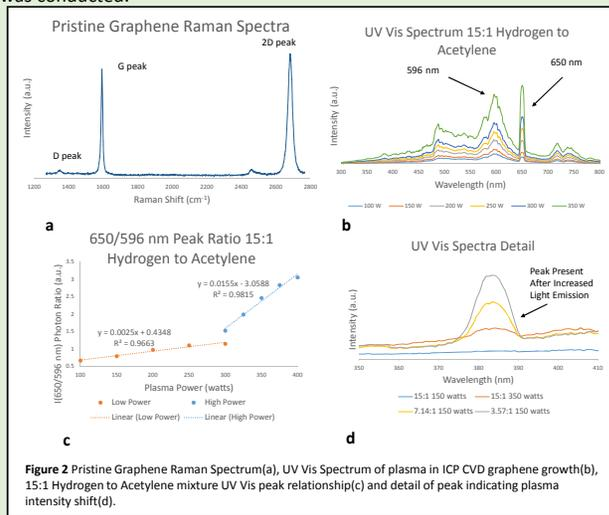
Figure 2 Pristine Graphene Raman Spectrum(a), UV Vis Spectrum of plasma in ICP CVD graphene growth(b), 15:1 Hydrogen to Acetylene mixture UV Vis peak relationship(c) and detail of peak indicating plasma intensity shift(d).
