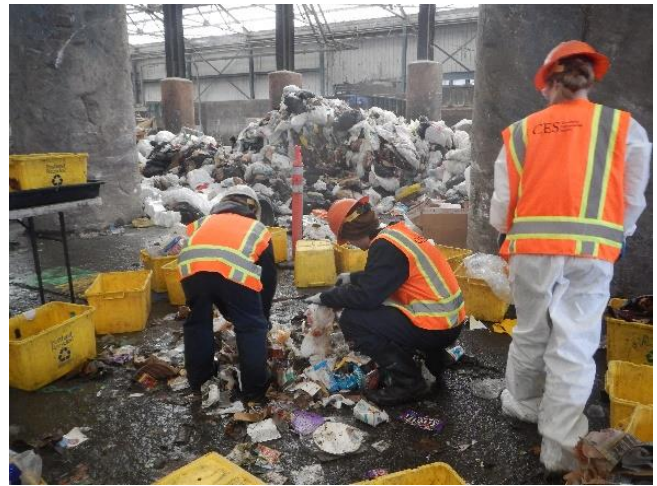
Image 2.2: Sorting method used for commingled recycling materials
