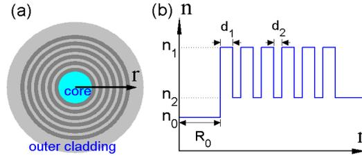
Fig. 1. Schematic of a Bragg fiber (a) and the radial index profile (b) (not to scale).
