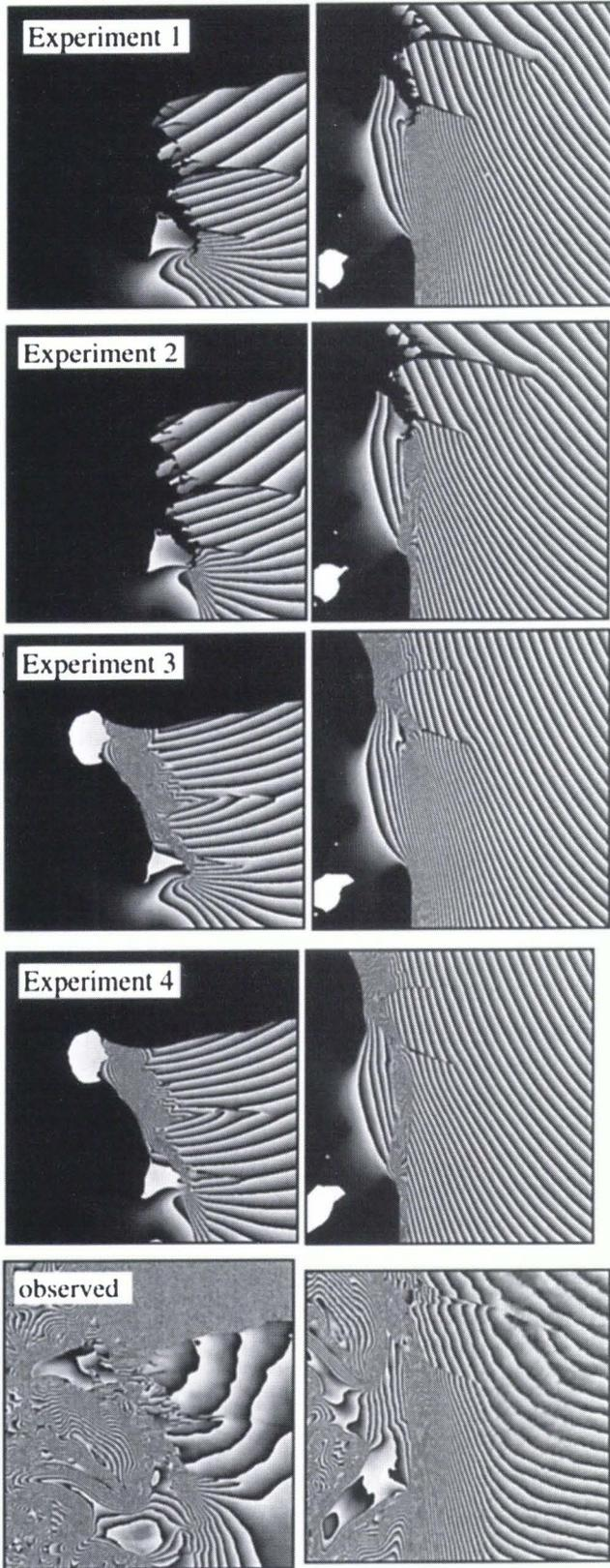
Fig. 4. Artificial and observed interferograms for the LC experiments. Descending satellite pass images are in the left-hand column, and ascending pass images in the righthand column. The best match between artificial and observed interferograms is for experiment 2, where a 50% coastal boundary-layer softening is applied and open-water rifts are assumed. The observed interferograms are from Rignot and MacAyeal (in press).
