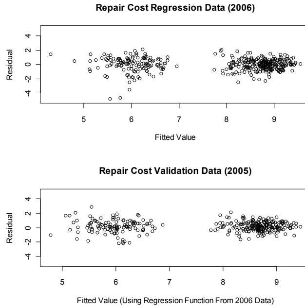
Figure 3.5 Repair cost residual plots for 2006 data (from the regression) and from 2005 data (after using the regression to predict costs).
