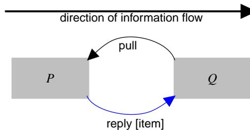
**Figure 1. The Pull model of data flow.**
