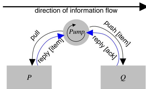
**Figure 3. An external *Pump* extracts data from *P* and pushes it into *Q***
