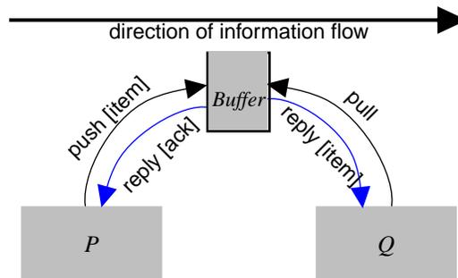
**Figure 4. An external *Buffer* receives data from *P* and supplies it to *Q***
