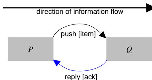
**Figure 2. The Push model of data flow.**
