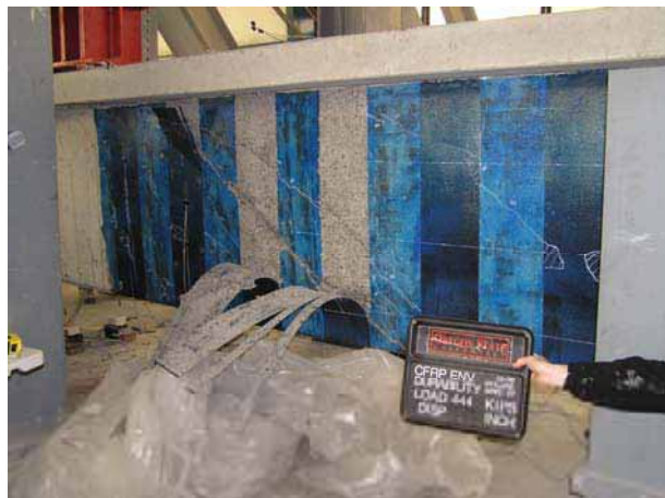
Figure 5.17: Failure photograph of Specimen T18Control
