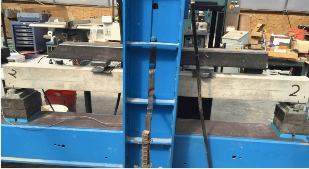
Figure 20: Testing beams using two-point loading
