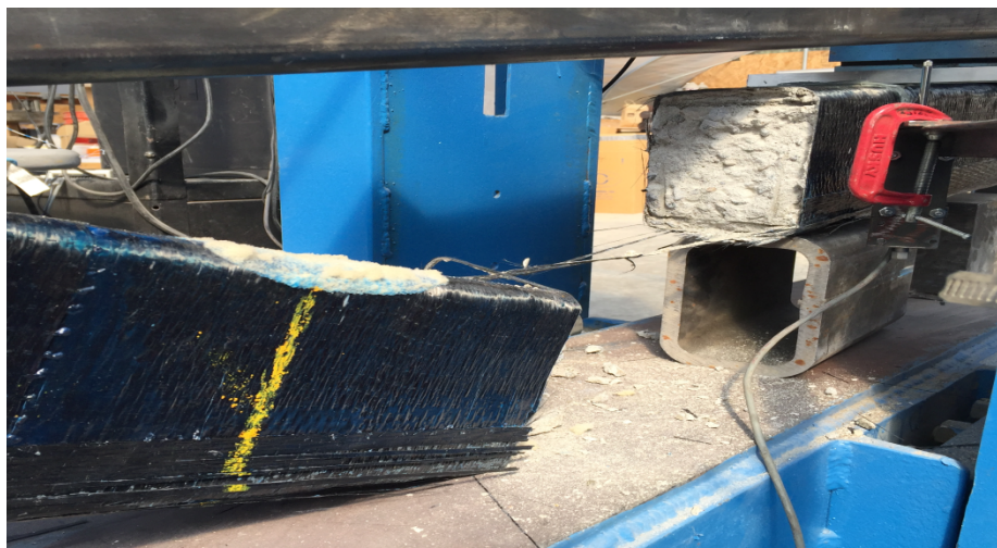
Figure 33: Combined rupture and brittle failure
