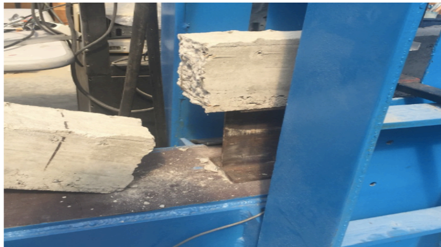
Figure 27: Beam #1 brittle failure
