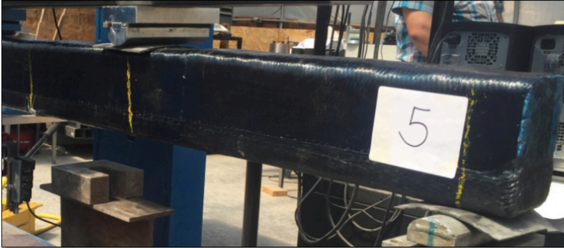
Figure 19: CFRP wrapped Beam #5
