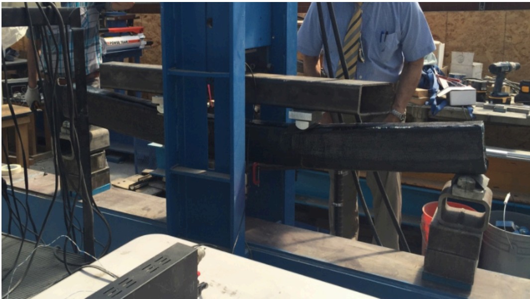
Figure 34: Beam #5 deflection capacity
