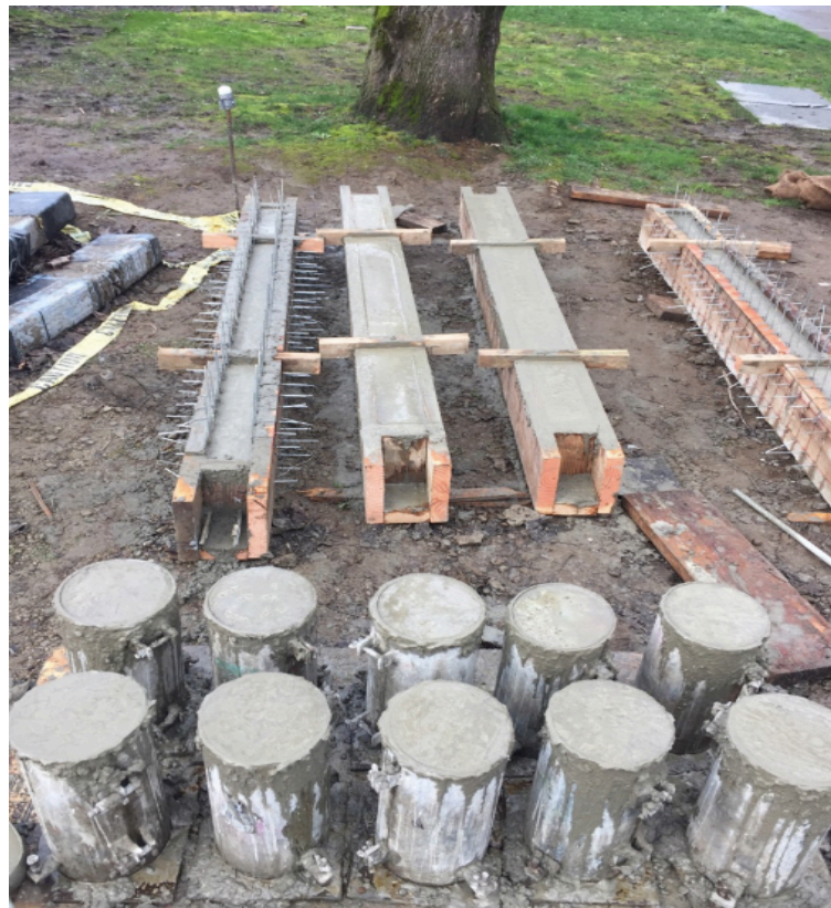
Figure 12: Concrete beams and cylinders
