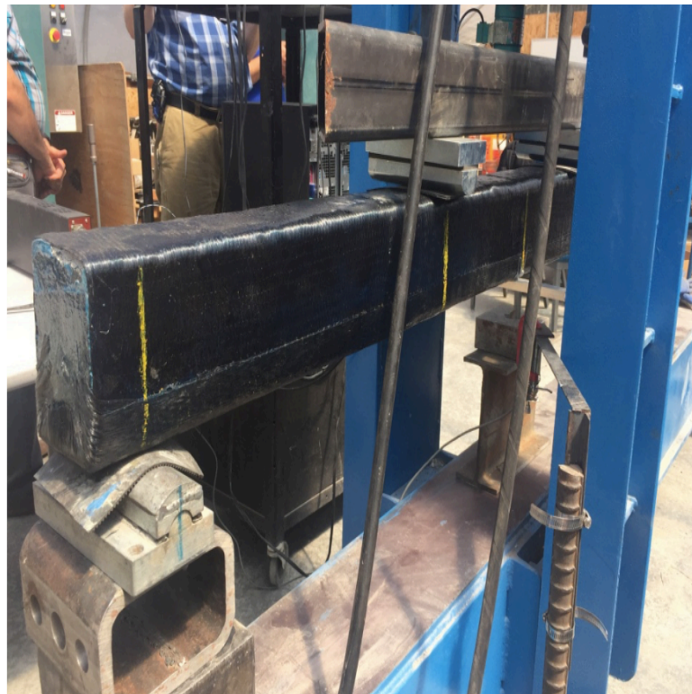
Figure 25: Testing CFRP-wrapped beam
