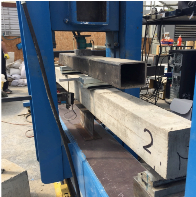
Figure 23: Beam test set-up
