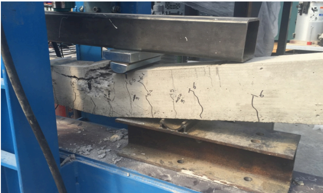
Figure 29: Concrete crushing in the compression zone
