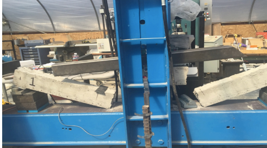
Figure 26: Failure mode of beam #1
