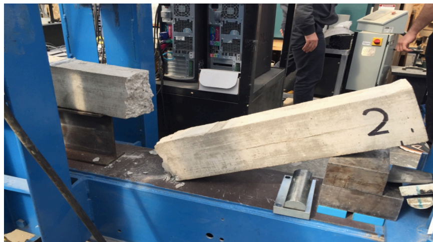
Figure 28: Beam #2 brittle failure
