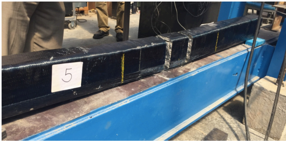
Figure 36: Beam failed half span distance
