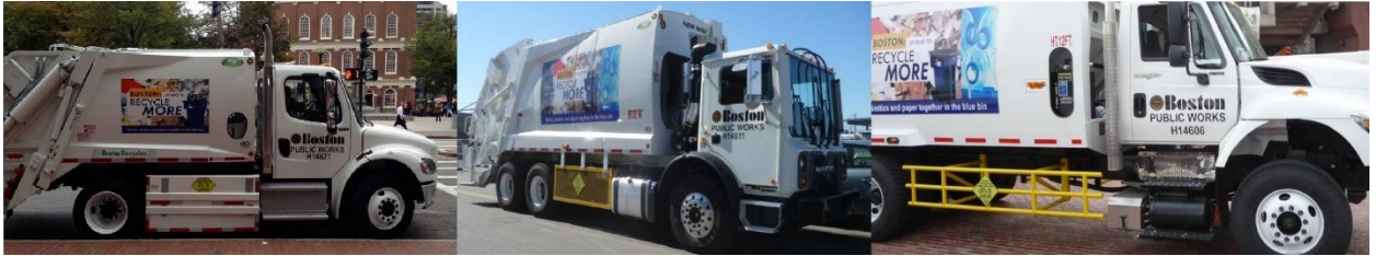
Figure 65. Various side guard styles on Boston Public Works vehicles
