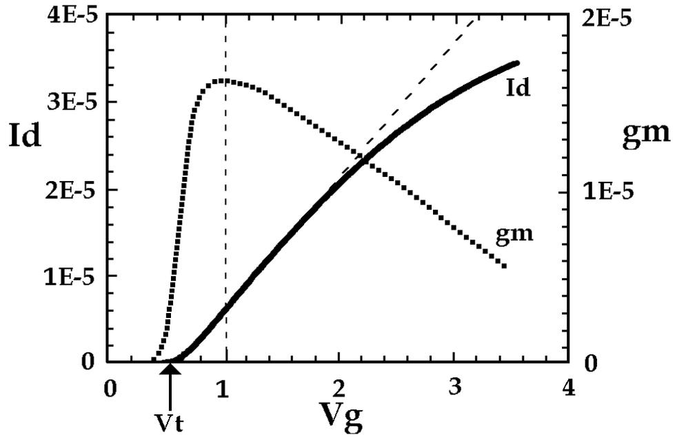
Figure 2.1 (after [1], Figure 4.24) - Transistor IV Curve With Transconductance
