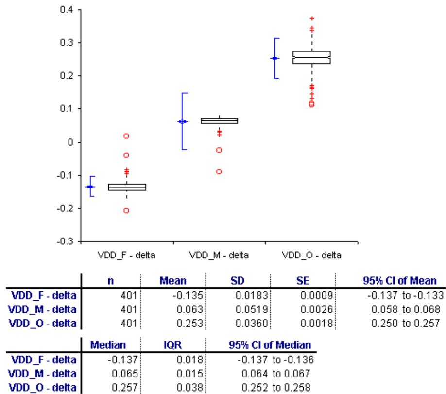
Figure 4.6 – ASIC1 MinVDD Temperature Shift Distributions
