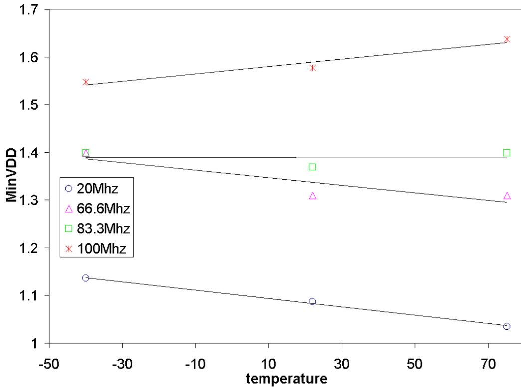
Figure 4.18 – ASIC2 LBIST MinVDD(Temperature) As Frequency Varies
