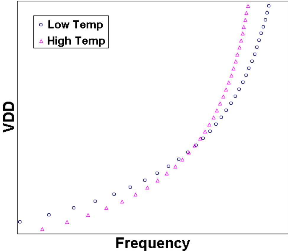
Figure 4.16 – Theoretical MinVDD( $f_{max}$ ) As Temperature Varies
