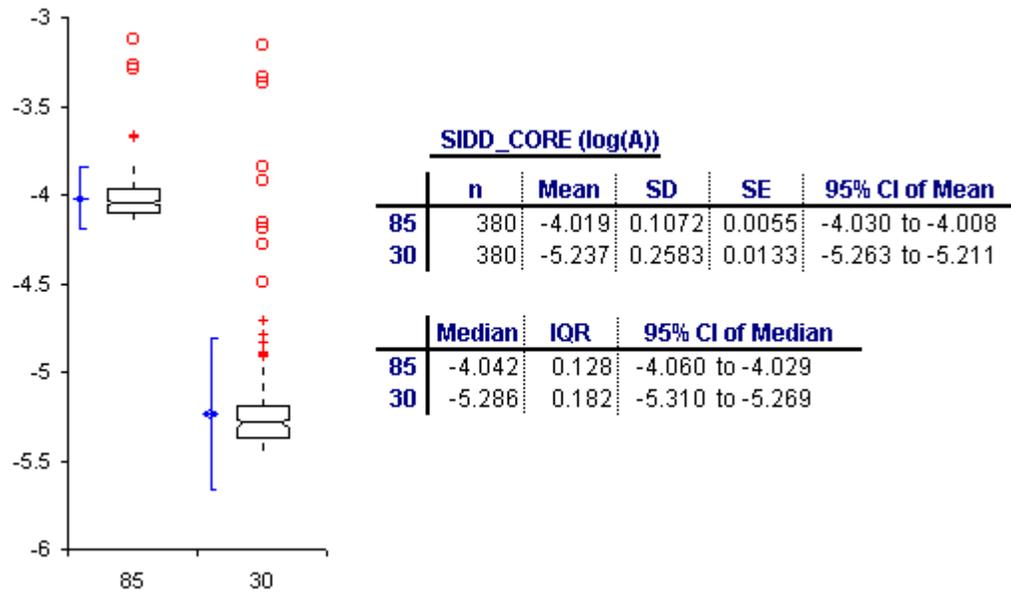
Figure 4.20 – ASIC1 Static IDD Distributions
