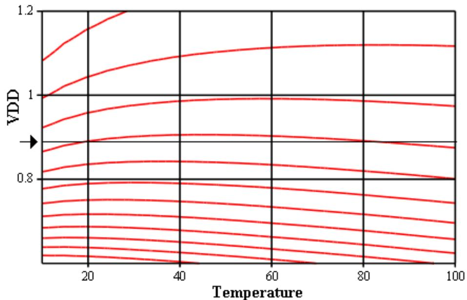
Figure 4.17 – Family Of MinVDD(T) Curves For 12 Fixed Frequencies
