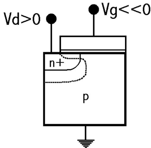
Figure 2.8 (after [6], Figure 2.46c) - Detail Of GIDL
