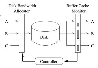
In this figure, the disk bandwidth allocator is multiplexing three real-rate streams (A, B, and C) based on allocations set by the controller. The buffer cache is monitored to track the progress of each stream. Stream A is below its target fill level, the controller will increase its proportion. Stream B is above its target, its proportion will be decreased. Stream C is on target, its proportion will be kept constant.
