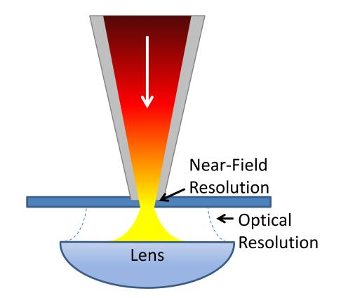
This limit can be overcome using near-field optical microscopy, in which light is delivered to the sample through a tapered optical fiber. In this case, the resolution is limited by the geometry of the tip. The illustration at left shows light incident on a sample from a near-field fiber probe, as compared with light from a lens in a traditional optical microscope.
