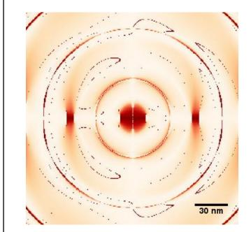
The results from FDTD are then fed to the algorithm to create a map of the Kerr rotation for a given sample and probe. An example from a typical nearfield probe is shown at left.
