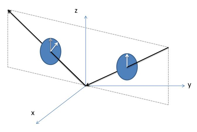
In the illustration (left), the light reflects from a magnetic surface. The direction of the magnetic field is initially straight up. Upon reflection, the field has rotated to its new position (shown by the white arrow).
