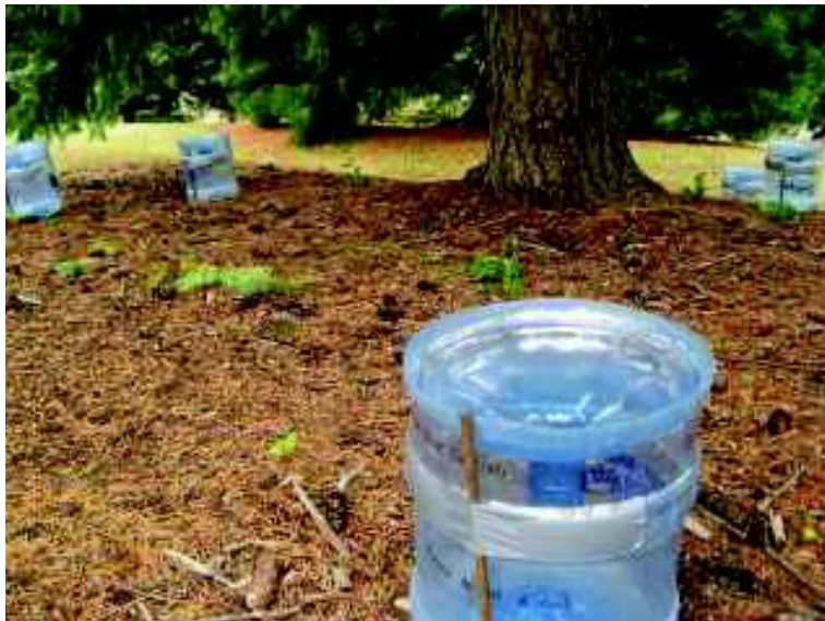
Figure 6. Photo of Buckets at Study Tree 4. The photo shows bucket placement and attachment to rebar stakes.
