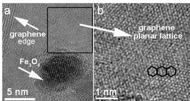
**Fig. 2** (a) HRTEM image of a graphene/ $\text{Fe}_3\text{O}_4$  hybrid prepared at  $180^\circ\text{C}$  for 8 h; (b) enlarged image of boxed area in (a).
