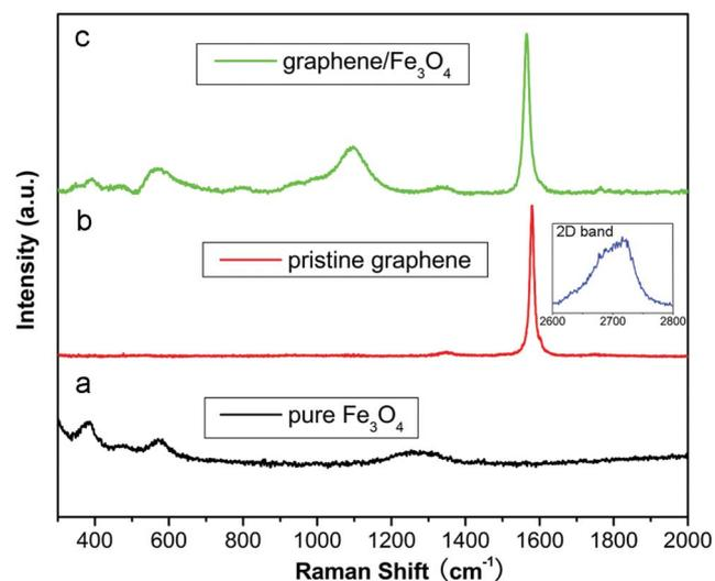
**Fig. 3** Raman spectra of (a) pure  $\text{Fe}_3\text{O}_4$  NPs, (b) pristine graphene and (c) graphene/ $\text{Fe}_3\text{O}_4$  composite.
