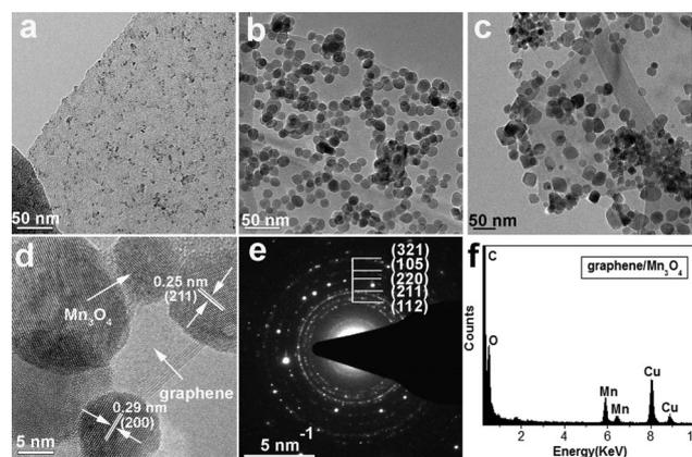
**Fig. 4** TEM analysis of graphene/ $\text{Mn}_3\text{O}_4$  composites prepared by solvothermal reaction at 200 °C. (a)–(c) show products prepared at reaction times of 4 h (a), 8 h (b), and 16 h (c), respectively; (d–e) HRTEM image of attached  $\text{Mn}_3\text{O}_4$  NPs (d) and the corresponding SAED pattern (e); (f) EDS pattern of the attached  $\text{Mn}_3\text{O}_4$  NPs.
