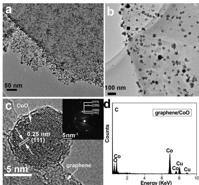
**Fig. 5** TEM analysis of graphene/CoO composites prepared by solvothermal reaction at 200 °C. (a)–(b) show products from reaction times of 8 h and 16 h respectively; (c) HRTEM image of deposited CoO NPs and the corresponding SAED pattern (inset); (d) typical EDS pattern of the deposited CoO NPs.
