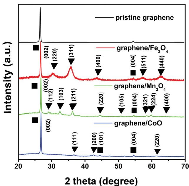
**Fig. 6** The XRD patterns of exfoliated pristine graphene, graphene/Fe<sub>3</sub>O<sub>4</sub>, graphene/Mn<sub>3</sub>O<sub>4</sub>, and graphene/CoO composites, respectively.
