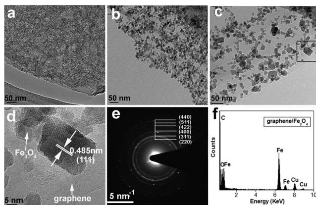
**Fig. 1** TEM analysis of graphene/ $\text{Fe}_3\text{O}_4$  composites prepared by solvothermal reaction at  $180^\circ\text{C}$  at varying reaction times of 4 h (a), 8 h (b), and 16 h (c); (d) HRTEM image of boxed area of (c); (e) the corresponding SAED pattern; (f) typical EDS pattern of the attached  $\text{Fe}_3\text{O}_4$  NPs.
