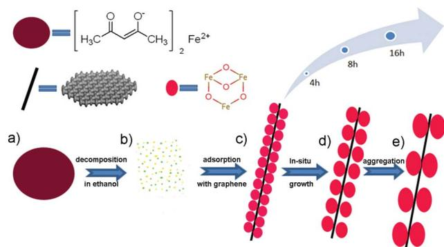
**Scheme 1** Schematic illustration of the whole reaction process: (a)  $\text{Fe}(\text{acac})_3$  precursor; (b) decomposition of  $\text{Fe}(\text{acac})_3$  into  $\text{Fe}^{2+}$  and  $\text{Fe}^{3+}$  cations; (c) initial nucleation of NPs and adsorption by graphene; (d) *in situ* growth to form monodisperse NPs on the surface of the graphene; (e) form larger NPs by Ostwald ripening.
