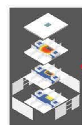
Building is exploded to display day light analysis grid.
