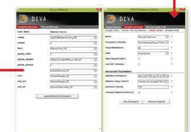
Material, time frame, and luminance settings are applied within Diva software options.
