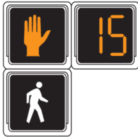
Figure 4-3: Pedestrian signal indications (Walking person, Flash Don’t Walk with count down display, and Solid Don’t Walk) (FHWA, 2009)
