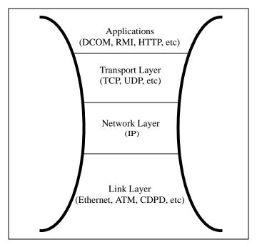
This figure shows the "hourglass" architectural model of the Internet. The waist of the hourglass is the ideal place to support mobility since it involves the least amount of change. The waist corresponds to the network level that consists of the IP protocol, which explains why most mobility research is focused at this level.
