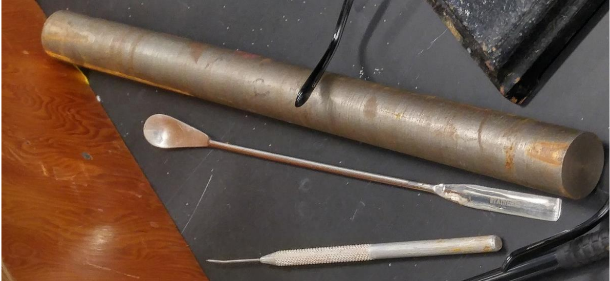
Figure 1: Tools used for packing columns. From top to bottom: tamping rod, scoop, and stylus.
