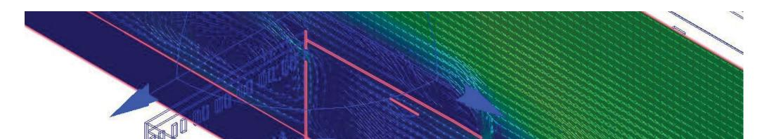
We ran iterative designs to determine the optimum air flow. We used a graphical representation of air speeds in the occupied zone to determine which designs produced the best airflow.
