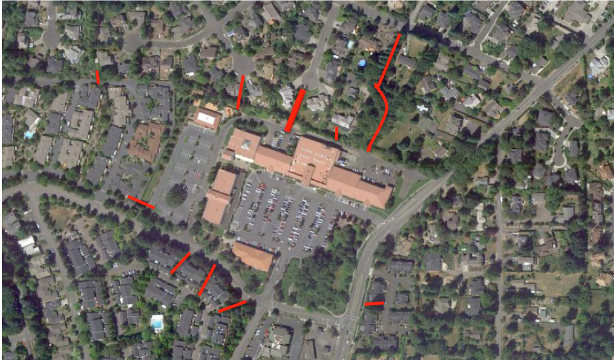
Figure 2: Informal Pedestrian Paths Around Oswego Town Center: Some of the paths are shortcuts into multifamily complexes, some connect through private land to the street network, and some are simply short paths and gates that connect only to a single private residence.
