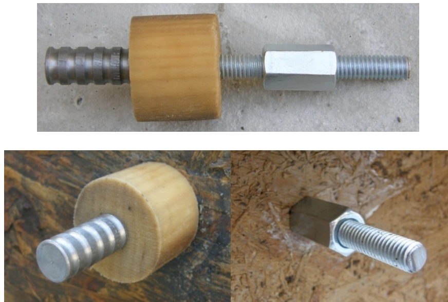
Figure 2-2: A) threaded steel insert assembly b) portion of the insert assembly on the inside of the form (left) and c) portion of the insert assembly on the outside of the form (right)
