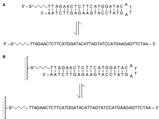
Figure 1. DNA hairpin melting reactions (A) DNA hairpin (containing 5' C 6 -thiol linker) in solution melts to a single strand. The temperature induced melting transition of the hairpin in solution was studied by DSC and UV absorbance versus temperature measurements. (B) DNA hairpin attached at the 5' end to gold electrodes via a C 6 -thiol linker. The temperature induced melting transition hairpin on the surface was monitored by measuring four distinct electronic properties of the molecule; Z, \theta , C and D, over a 10 6 frequency range at different temperatures.
