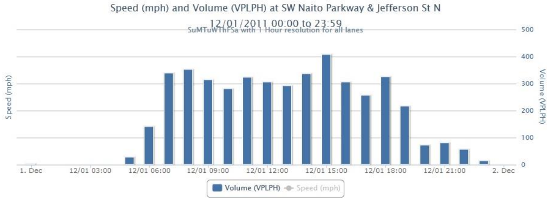
Figure 7.5 Volume Plot (One-hour Resolution)
