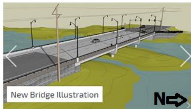
Figure 9: Artistic rendition of new four lane open span bridge with two creek channels. Courtesy of Kitsap County Public Works: Bridge Illustrations
