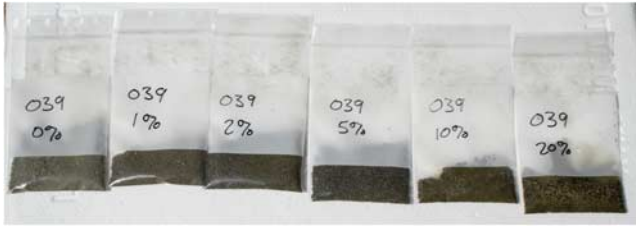
Fig. 3. Sediment samples prepared for analysis. Based on visual inspection alone, it is very difficult to discern differences in soil colour and texture based on water content. Most darkening occurs in the first few weight percent of water. Sample bags are c. 8 cm wide.
