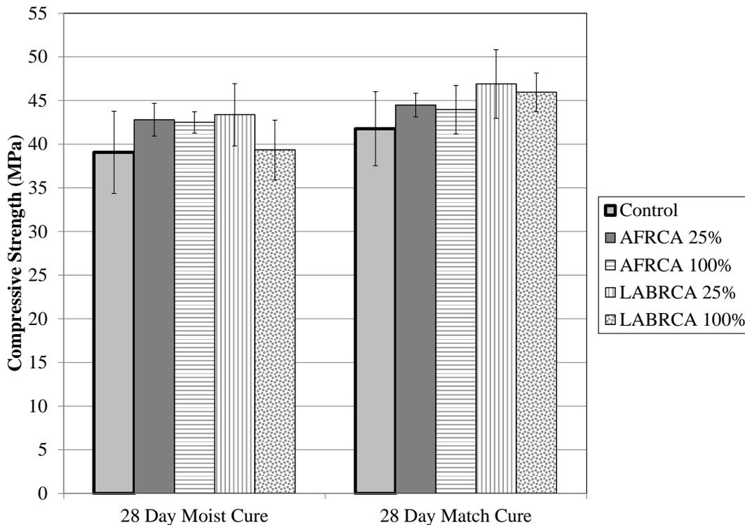
Figure 3.1: 28-day compressive strength for concrete mixtures
