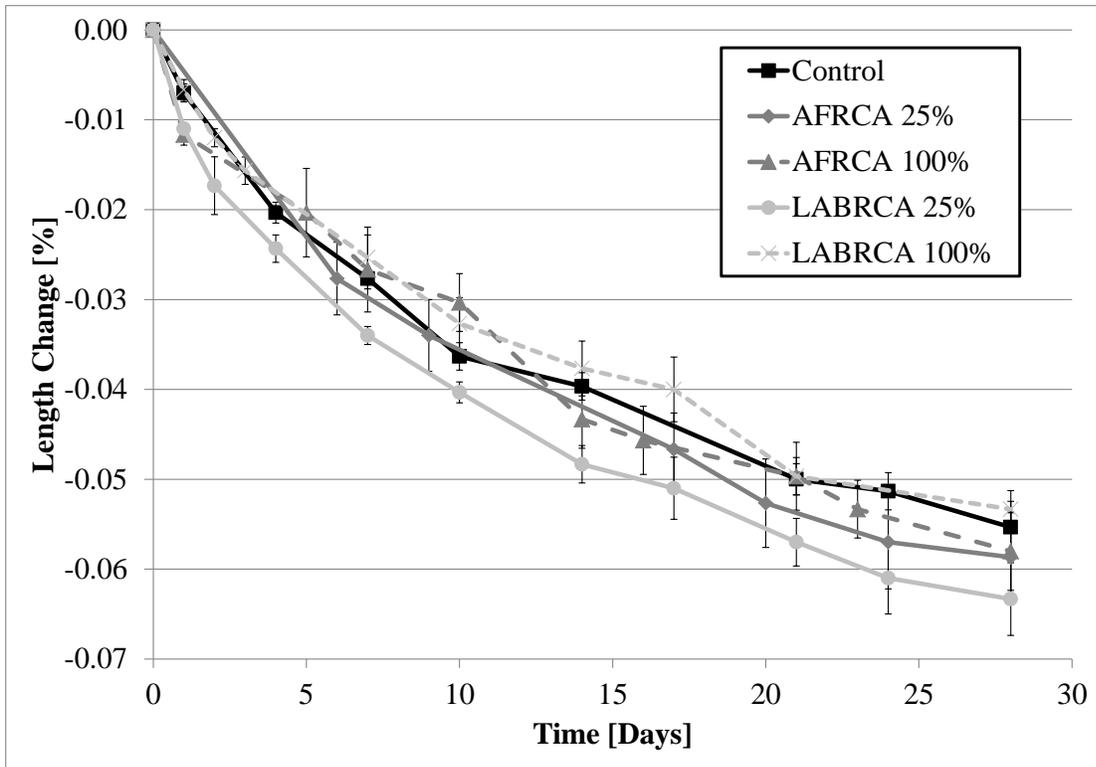
Figure 3.4: Drying shrinkage over time for concrete mixtures
