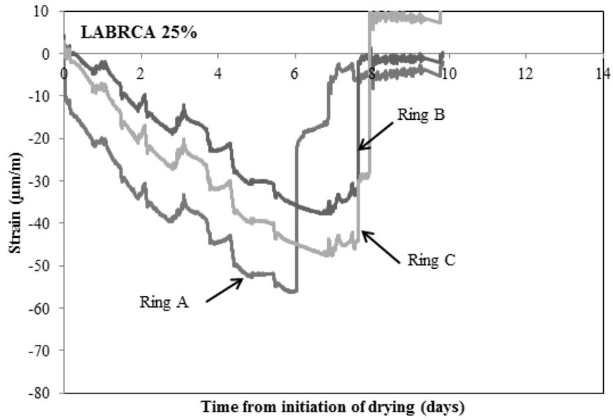
Figure 6.7: Strain gauge reading of mixture LABRCA 25%
