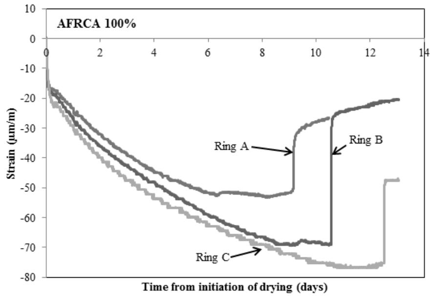
**Figure 6.6: Strain gauge reading of mixture AFRCA 100%**
