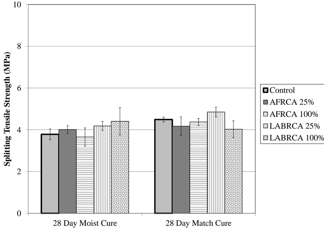
**Figure 3.2: 28-day splitting tensile strength for concrete mixtures**
