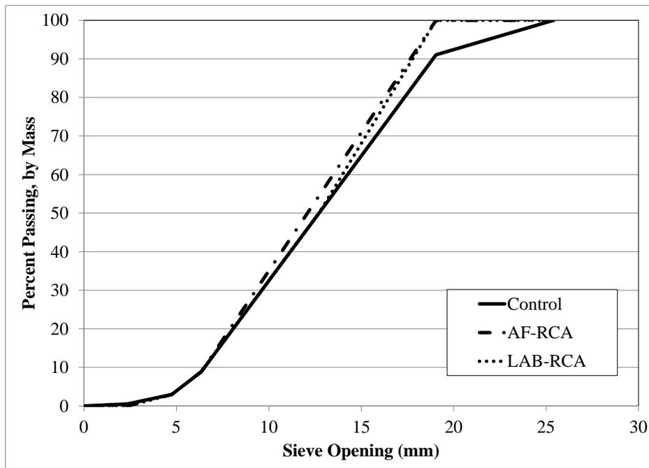
**Figure 2.1: Coarse aggregate grading**
