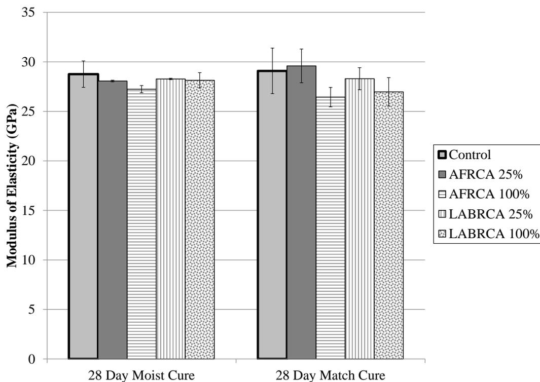
Figure 3.3: 28-day moduli of elasticity for concrete mixtures
