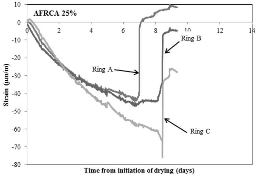
**Figure 6.5: Strain gauge reading of mixture AFRCA 25%**
