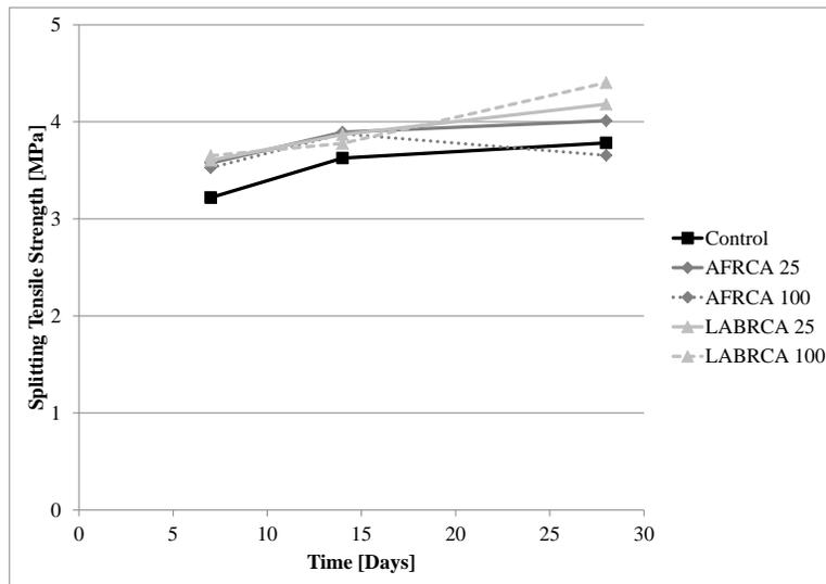
**Figure 6.2: Splitting tensile strength of concrete mixtures**
