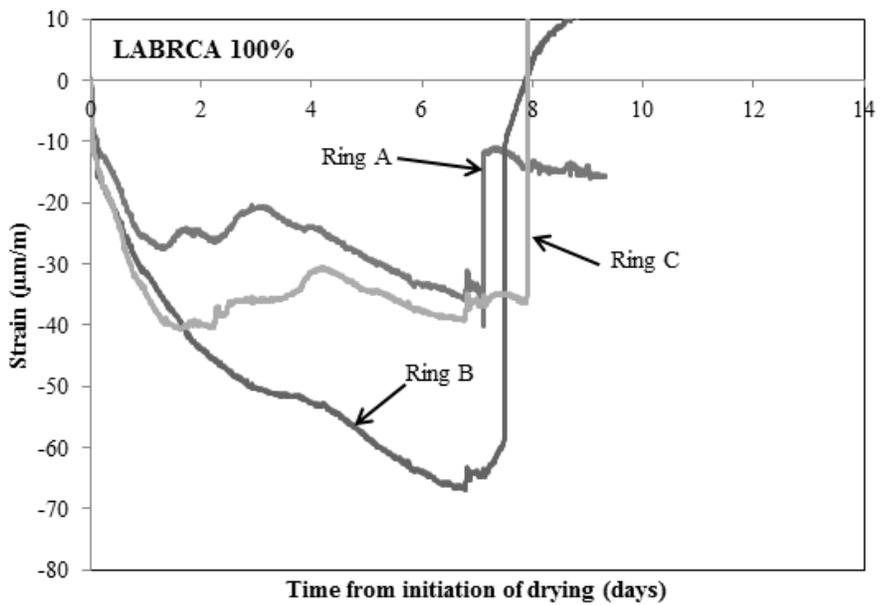
Figure 6.8: Strain gauge reading of mixture LABRCA 100%
