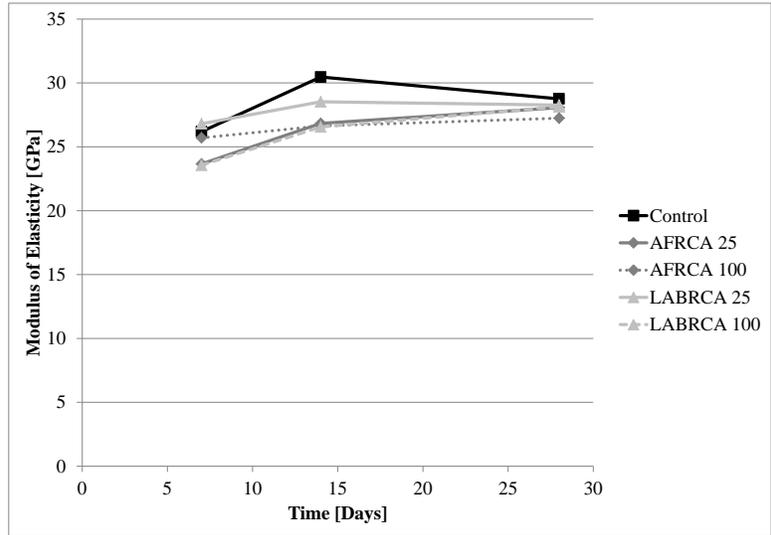
Figure 6.3: Modulus of elasticity of concrete mixtures
