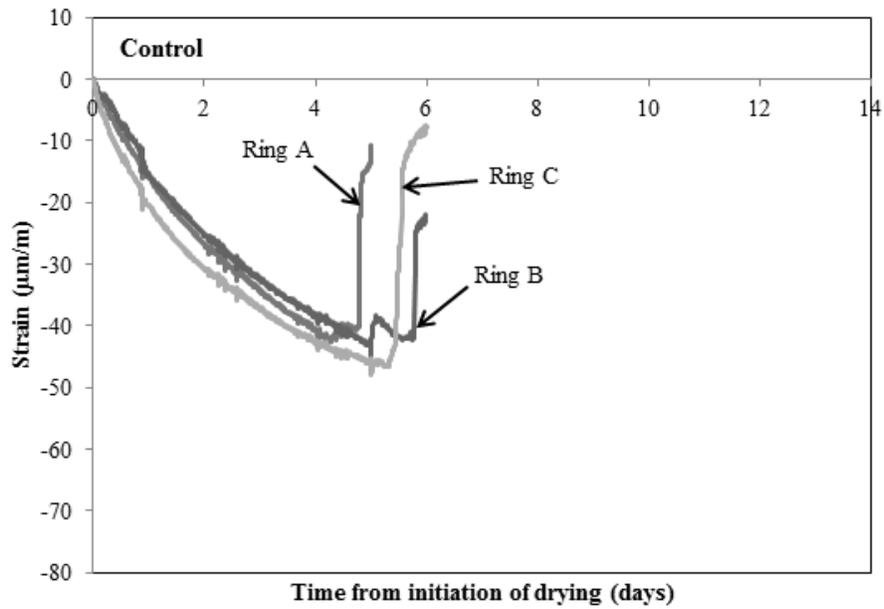
Figure 6.4: Strain gauge reading of mixture control
