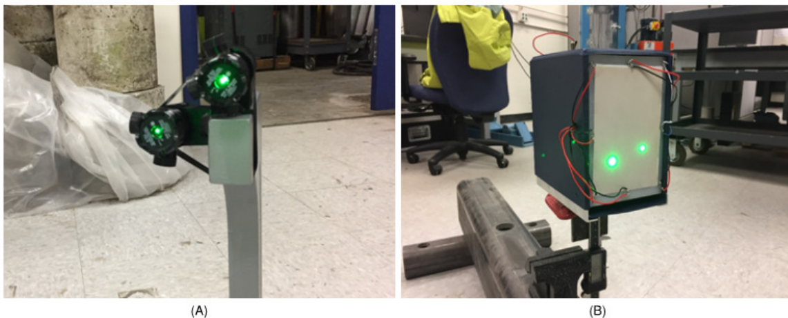
FIG. 6 PHOTO OF SENSOR PROTOTYPE: (A) FIXED AND (B) MOVABLE PART OF THE SENSOR USED IN LABORATORY STUDY 1
