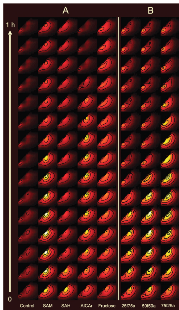
Fig. 4. Time and wavelength dependent detection. (A) EEMs of control and 1 plus 100 \mu\text{M} of analyte. (B) EEMs of 1 plus fructose and AICAr mixtures. Total concentration of each analyte mixture is 100 \mu\text{M} . The ratio of fructose to AICAr is increased toward the right as indicated. The first EEM in time is plotted at the bottom with time increasing toward the top. Experimental conditions as well as excitation and emission axes correspond to those in Fig. 2.
