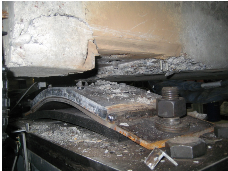
Figure 21: Failure of specimen HS-1.
