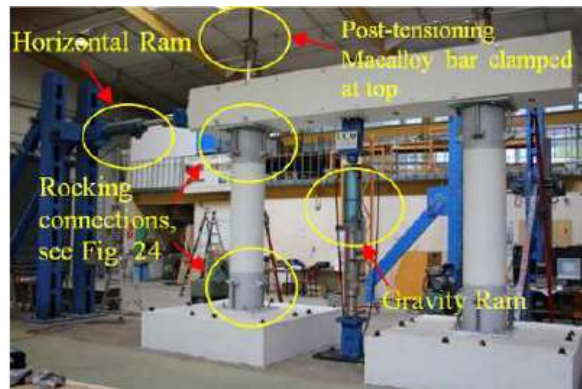
Figure 2.7: Testing configuration (Mashal, Palermo, & Chegini, 2014)
