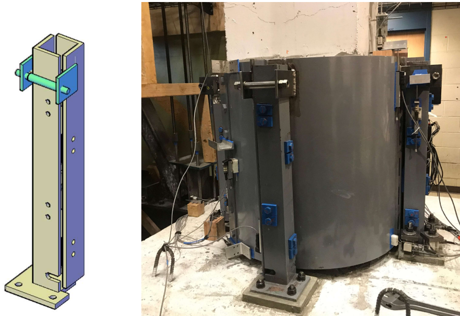
Figure 5.16: Test 3 modification - hold-down roller
