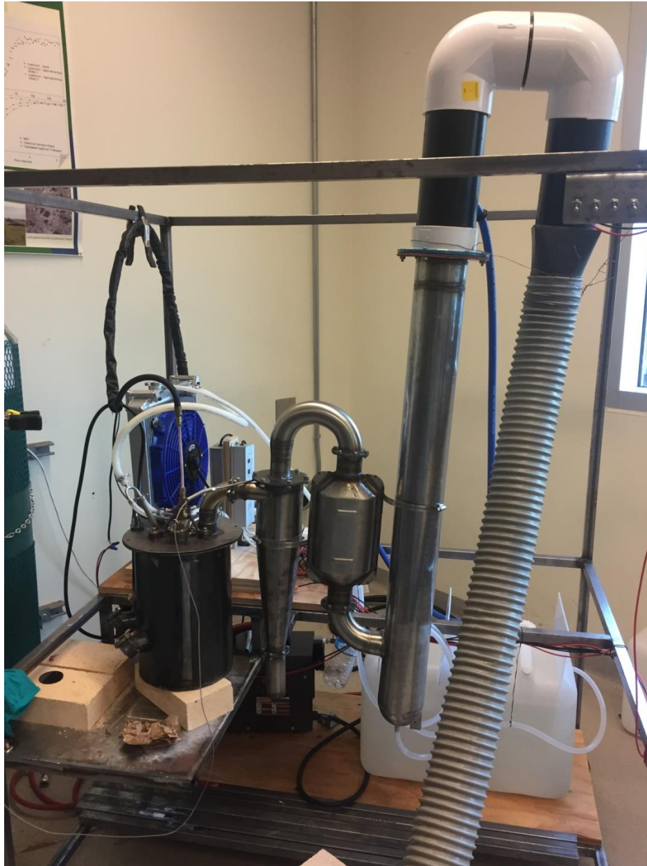
Figure 10: Prototype plasma gasification system in the lab.
