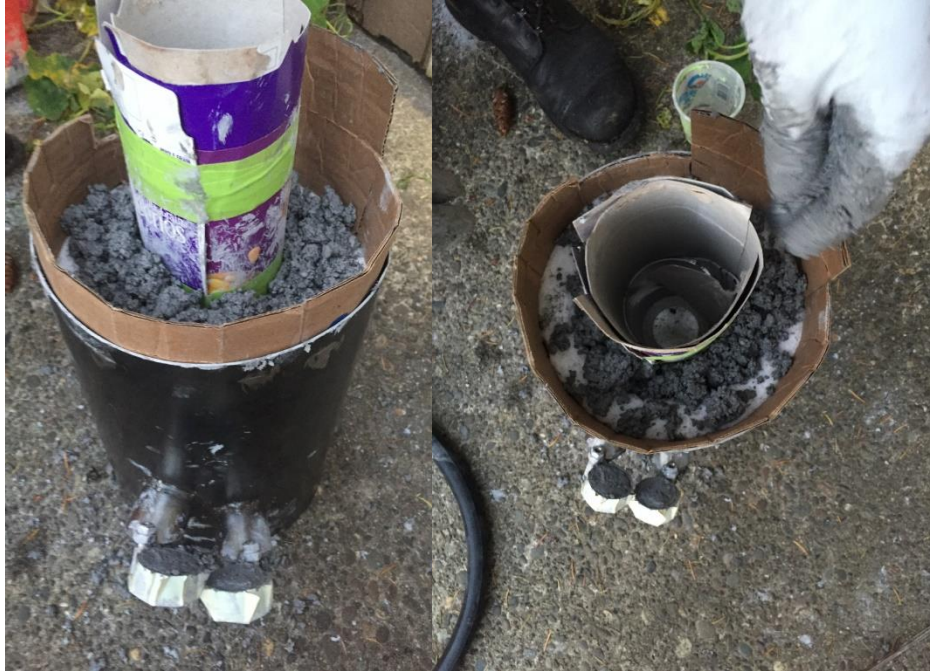
Figure 25: Gasification chamber being filled with refractory cement.
