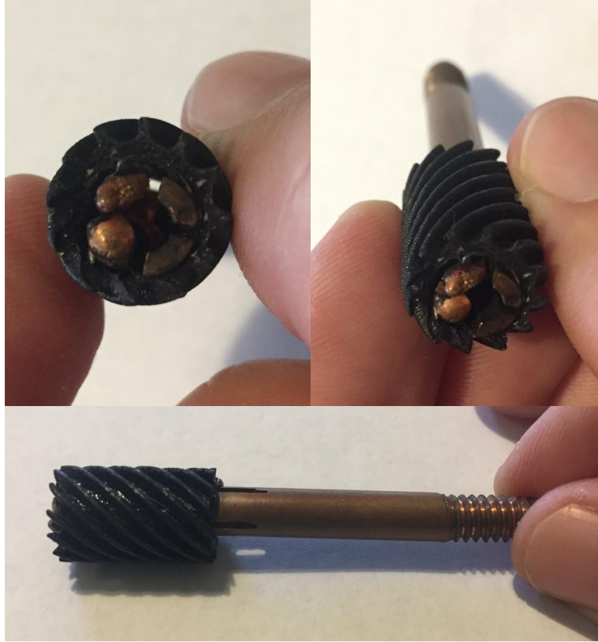
Figure 19: Melted vortex generator and collet.
