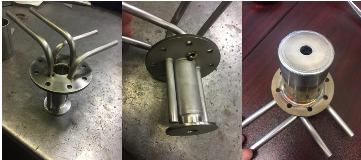
Figure 14: Coolant jacket for the plasma torch. Inlet and outlet tubes connected to the flange (left), internal view of the torch tube, coolant tube connections and end piece (middle) and the gasification side of the completed jacket (right).
