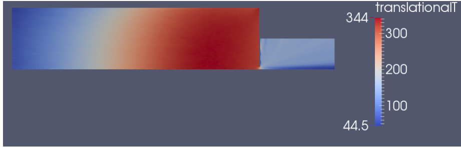
Figure 3-7: A heatmap of the translational temperature for helium atoms at each point in a 2 \mu\text{m} half-width simple slit. This plot shows the simulation reflected across the y axis to show the full skimmer operation. Helium gas flows from the left isotropically with a number density of 5 \times 10^{22} , an average velocity of 1750 m/s and an initial temperature of 1 K.
