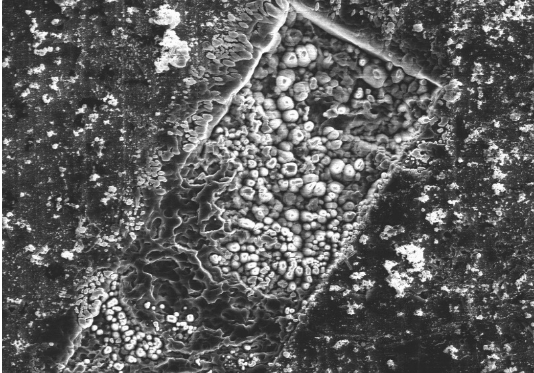
Figure 23: SEM picture of a milling pattern made with high energy ion beam. The pattern is 50 \mu\text{m} in width.
