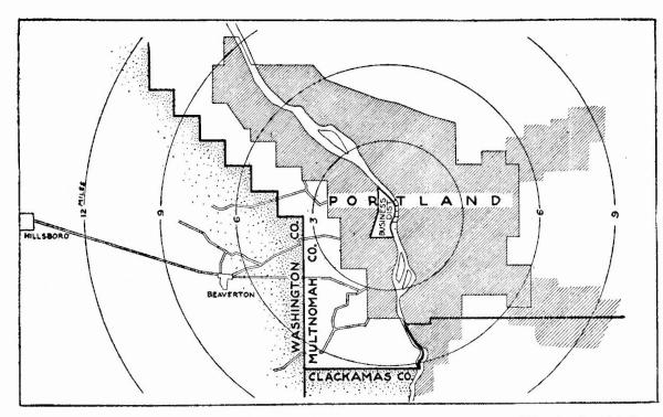
Map showing overlapping political jurisdictions paralleling the hills west of Portland which have made the construction of high class traffic arteries in that direction impossible thus forcing new development east of the river. Some of the newer residential sections are nine miles or more from the west side business district. This unbalanced development results in increasing traffic congestion on our TransWillamette river bridges.
