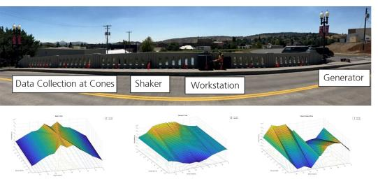
The frequencies associated with each of these plots are 7.80 Hz, 11.70 Hz, and 15.00 Hz, respectively. For more detail, download the final report.
