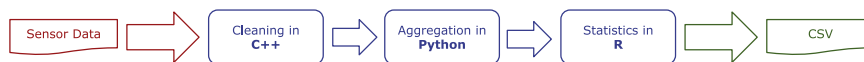
Fig. 3. Title: Workflow combining different programming languages. Description: this figure illustrates an example workflow that processes data using different programming languages.
